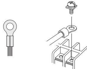
**⚠** It is compulsory to use ring crimp terminals to connect to the terminal board.
