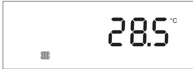
Example of display on stand-by (outdoor probe is connected).
