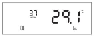
The demand is activated when the room/heat demand thermostat's contact is closed provided that outdoor temperature does not exceed the value set by the parameter 2025. if the outdoor temperature is higher than the one set on parameter 2025, the burner is stopped even if there is a heat demand.
