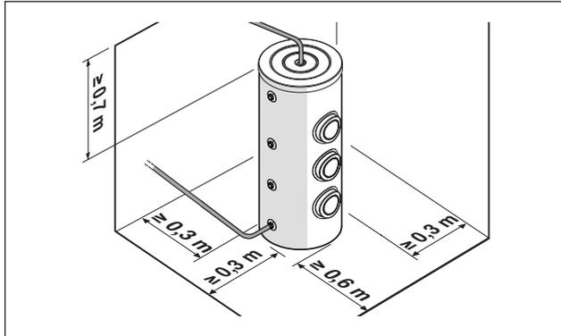
**NOTE:** the above-indicated dimensions are recommended for a correct maintenance and access to the device.
