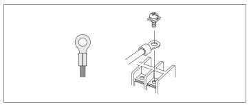
$oldsymbol{\Lambda}$  It is compulsory to use ring crimp terminals to connect to the terminal board.
