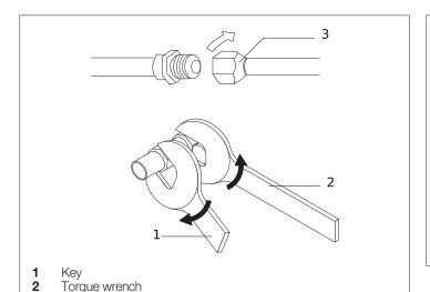
Pipe Ø **Tightening torque** inches Nm mm 6.35 1/4 18 9.52 3/8 42 12.7 1/2 55 15.88 5/8 60
