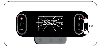
second press set CH setpoint value in steps of 0.5 °C
