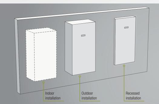
CIAO S has been specifically designed to be installed also outdoor in partially protected or recessed places, thanks to the specific accessories and the frost protection kit down to -10°C (available as option). Upper and lower covers are also
