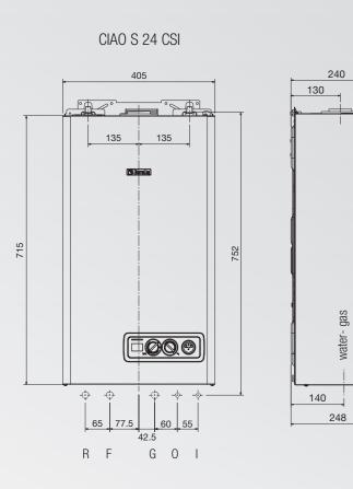
KEY: System: Return R/ Flow F/ Gas G Domestic water: Inlet I/ Outlet 0
