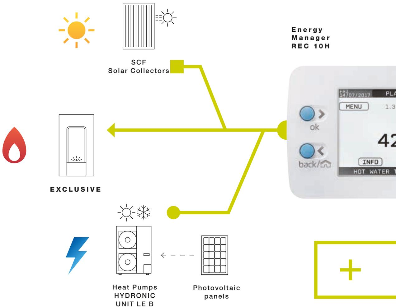
Provided with a new communication BUS, EXCLUSIVE is able to interact perfectly with the Energy Manager REC 10H, the “brain” of the system, which can constantly monitor the hybrid system in order to provide the best home comfort.
