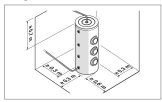
NOTE: the above-indicated dimensions are recommended for a correct maintenance and access to the device.
