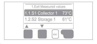
If the cables are too long or the sensors not positioned correctly, there could be minor deviations in the measurement values. In this instance, the values displayed can be compensated by making adjustments via the controller. The temperature measured is the temperature at the outlet of the heat exchanger, which could differ from that measured at the user points. Small fluctuations in temperature at the user points are compensated generally by mixing water from the main.
