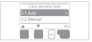
ing a mains power failure, the controller will revert automatically to the operating mode last selected!
