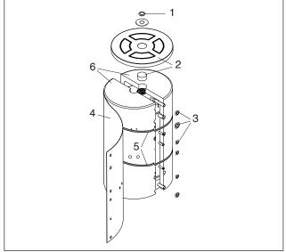
igtarrow Make sure that the insulation shells (7) are securely fixed in place by straps before fitting the plastic cover. Use a strap wrench if necessary.
