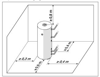
Respect the minimum specified installation distances to ensure correct installation and access for maintenance.
