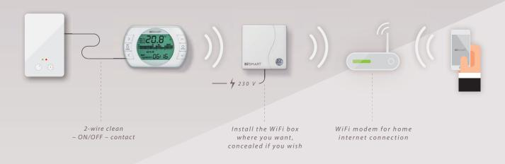
**NB:** When replacing a thermostat that has more than two wires, identify the 'switch' wires and connect only them to the BeSMART ON/OFF terminals (do not connect a Neutral supply to BeSMART). The BeSMART control is powered by 2 AA batteries; it therefore does not require a fixed 230 V mains power supply.
