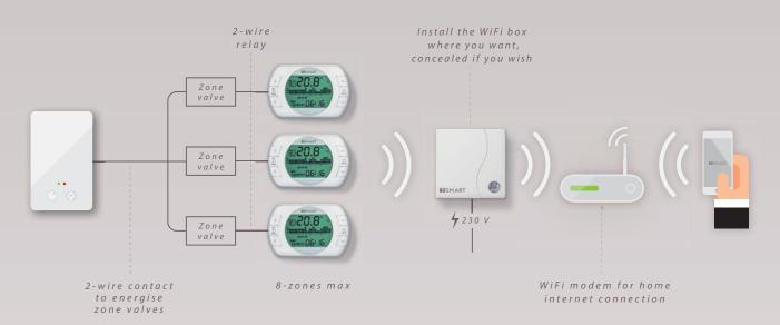
**NB:** When replacing a thermostat that has more than two wires, identify the 'switch' wires and connect only them to the BeSMART ON/OFF terminals (do not connect a Neutral supply to BeSMART). The BeSMART control is powered by 2 AA batteries; it therefore does not require a fixed 230V mains power supply.
