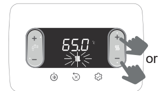
second press set CH setpoint value in steps of 0.5 °C
